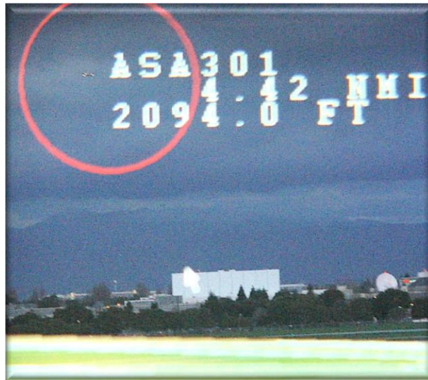
Data block and the circle are projected on aircraft
