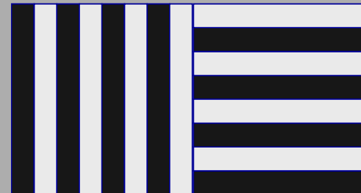
Optical line pair (OLP) test pattern
