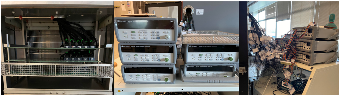
Fig. 14 Experiment setup for in situ measurement of resistance change
