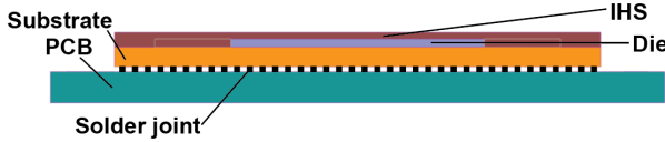
Fig. 6. Schematic of the BGA package.
