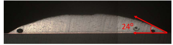
Fig. 2. SAC305 solder paste contact angle measurement.
