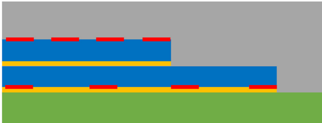
Fig. 14. Horizontally distributed initial cracks at material interfaces.
