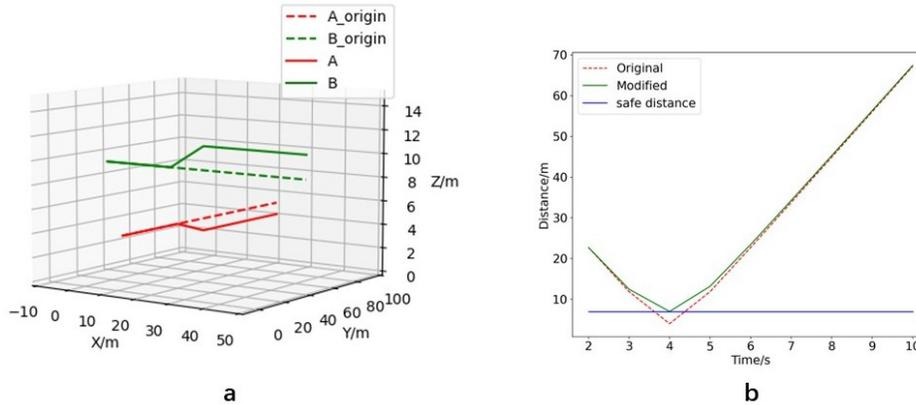
**Fig 5** (a) 3D trajectories of both UAVs. (b) Relative distance compared to  $D_{safe}$
