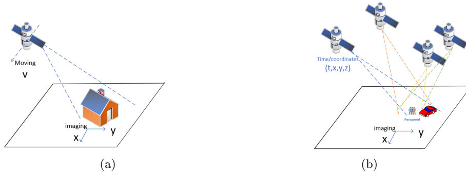
Fig. 1. (a) Conventional single-satellite SAR imaging. (b) Proposed LEO satellite constellation imaging (LEOSCI) with high resolutions to sense small targets.
