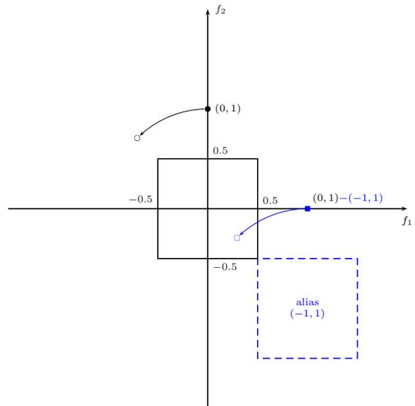
**Figure 5: Characteristic peaks as a result of aliasing for 2D resampling (counterclockwise rotation of  $45^\circ$ ). Characteristic peak in the baseband (solid square) originates from high frequency alias  $(-1, 1)$ .**
